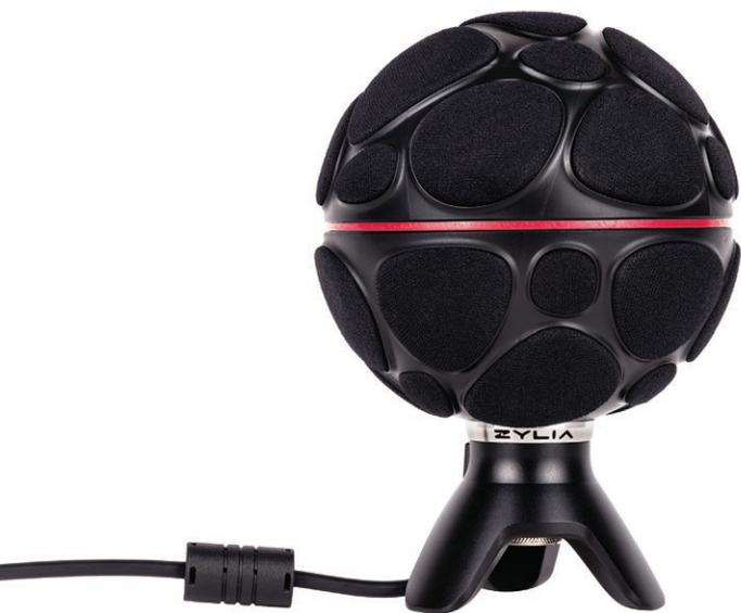
From M/S we go to first-order ambisonics, with four mic capsules generating raw signals that can be decoded into loudness, side-to-side, and front-to-back, but with no height information. Second-order ambisonics takes 8 mics, and third-order takes 16; the more mics and math, the more accurate the 3D representation.
